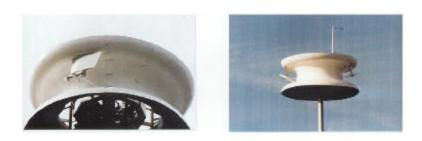
Turbines: Two 3 ft. diameter rotors Total Rating: 1.5 kW for battery charging
