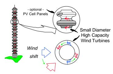
Fig. 1a. WARP Modules Amplify Wind to 80% & Yaw into Wind
