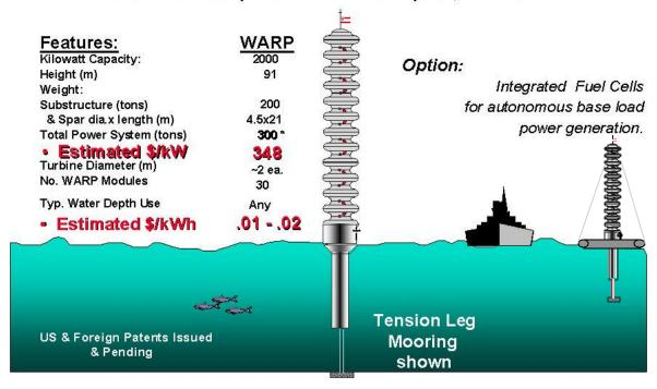
Figure 8. A Spar-WARP Power System Can Be Flexibly Deployed & Operated in Any Depth Water (not to scale)
