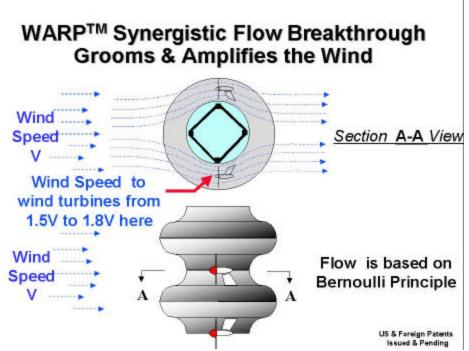
Fig. 1b WARP Module Flow Enhancement to Turbines is based on Bernoulli Principle
